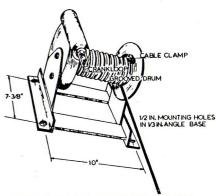
THIS WINCH IS A COMPLETE ASSEMBLY ON A EASY TO USE MOUNTING FRAME. IT HAS A 40 TO 1 RATIO WORMGEAR AND IS ENGENEERED TO.ILAST. THE CRANKLOOP IS DETACHABLE FOR REPLACEMENT IT COMES WITH A BUILD IN CABLE CLAMP FOR 3/6' STEEL CABLE. THIS UNIT IS TO BE OPERATED WITH A CRANK HAND WINDER.
